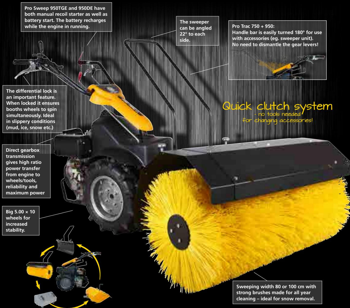
Pro Sweep 950TGE and 950DE have both manual recoil starter as well as battery start. The battery recharges while the engine is running.
